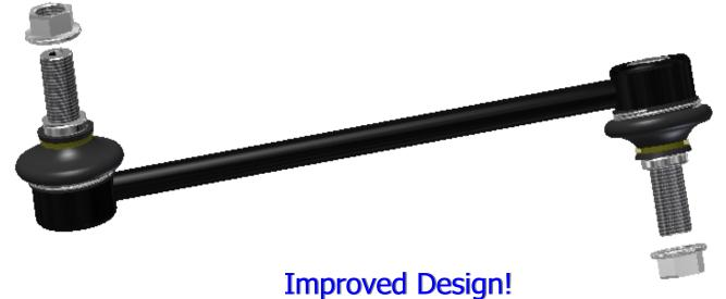
Heavy duty design for rugged condition. Bigger ball stud than OE Sealed boot design to eliminate contaminants from entering the bearing surfaces. Wrench flats & Hex Sockets for trouble-free installation & installer satisfaction.
