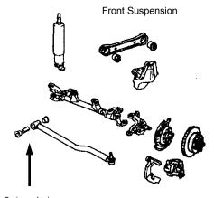
2 piece design bushings allow for easy installation.
